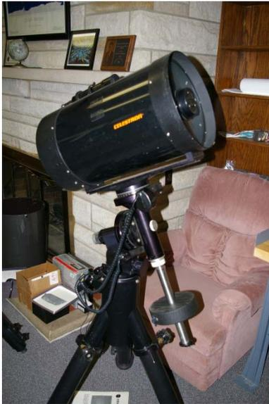
Telescope 2: 11-inch Schmidt-Cassegrain telescope made by Celestron on a CG mount. This mount is a “go-to” mount. Telescope comes with documentation, star diagonal, eyepiece, solar filter, padded storage box and power supply and battery. Minimum bid: \$600.
